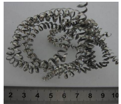
P = 100\text{ bar} , a = 1\text{ mm} , V_c = 50\text{ m/min} , f = 0.15\text{ mm/rev}
