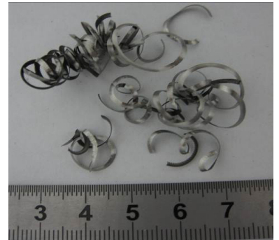
P = 300\text{ bar} , a = 1\text{ mm} , V_c = 50\text{ m/min} , f = 0.05\text{ mm/rev}
