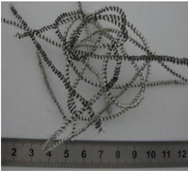
P = 100\text{ bar} , a = 0.5\text{ mm} , V_c = 50\text{ m/min} , f = 0.10\text{ mm/rev}
