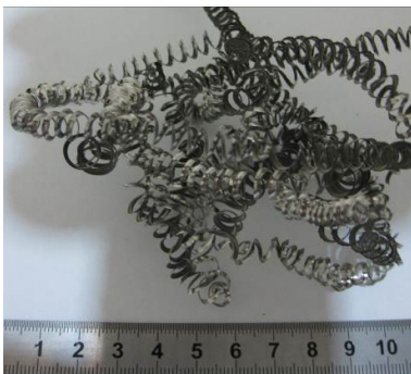
P = 6\text{ bar} , a = 1\text{ mm} , V_c = 70\text{ m/min} , f = 0.15\text{ mm/rev}
