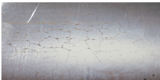
Figure 9: Stall band firecracks at the work roll surface.
