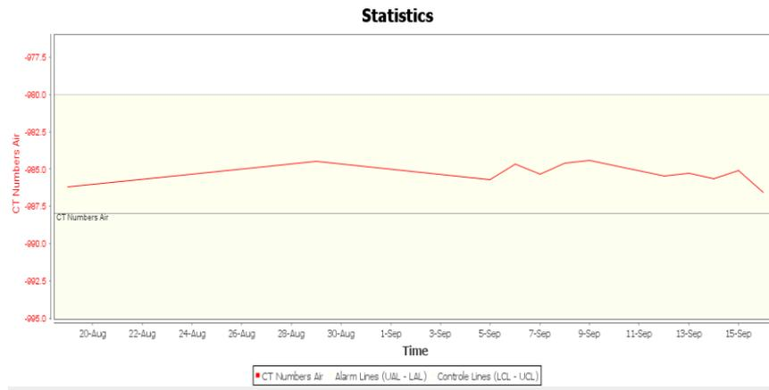
**Picture 4.** The graphical display of the values of CT air numbers during the considered period did not exceed the limit values of  $\pm 20$  HU.
