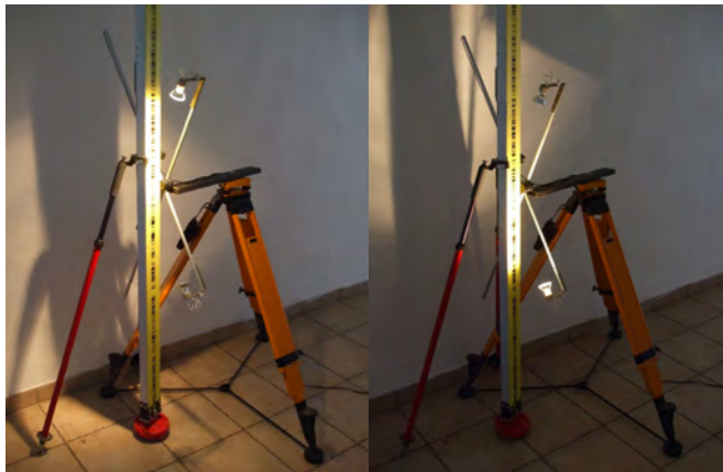
Figure 6: Illumination of the bar code; left - from above, right - from below.
