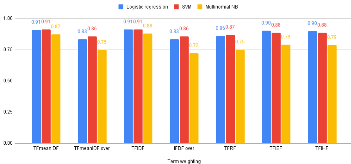
Figure 8: Comparison of Micro average of F1 score obtained from various term weighting methods (Experiment C Long text classification problem).
