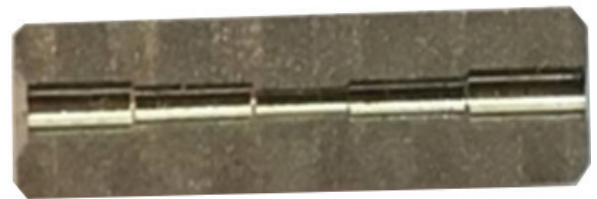
Fig. 17. Physical diagram of the 5 th order variable-diameter pipe after cutting
