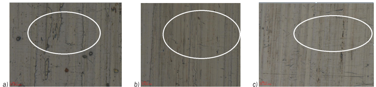
Fig. 7. Optical microscopic views of finished surface; a) with DC power supply without pulse, b) with pulse DC power supply at 0.27 duty cycle, c) with pulse DC power supply at 0.16 duty cycle
