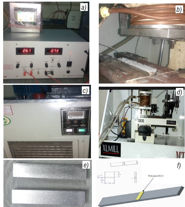
Fig. 1. a) Pulse DC power supply, b) BEMRF tool with MR fluid on workpiece, c) chiller for cooling the electromagnetic coil, d) BEMRF setup, e) EN-31 finished workpiece, f) schematic of die with workpiece dimension in mm
