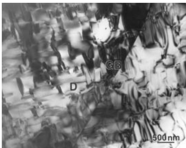
Fig 2: TEM micrographs of a \text{CaTiO}_3\text{-NdAlO}_3 sample: area near the grain boundary (GB) showing the presence of domains (D).
