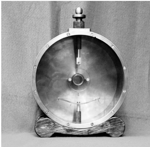
Reproduction of Wulf electrometer used by V. Hess to discover the existence of cosmic rays using a balloon (model built by INFN Padova)
