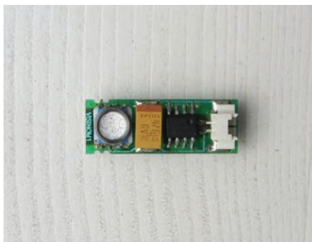
Višinomer, komponentna stran (9,0 x 22,0 x 9,0 mm, <2,5 g z baterijo)
