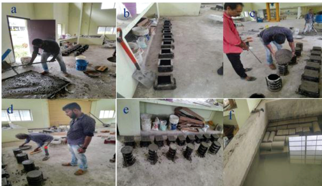
Figure 2: Preparation of: a) conventional concrete, b, c, d, e) green concrete cubes and cylinders, f) Concrete cylinders and cubes cured in a curing tank for (7, 14 and 28) d
