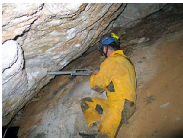
Fig. 2: Pološka Jama, TM 71 monitoring between two limestone beds dipping towards SE (Photo: S. Šebela).
