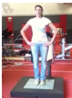
Figure 1. The position of the subject on the force platform.
