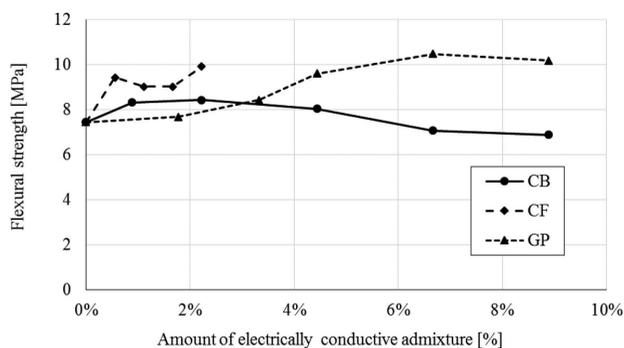
**Figure 7:** Flexural strength of electrically enhanced AAAs
