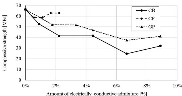
**Figure 8:** Compressive strength of electrically enhanced AAAs
