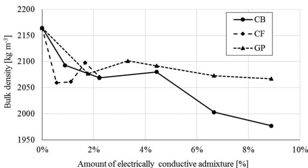
**Figure 4:** Bulk density of electrically enhanced AAAs
