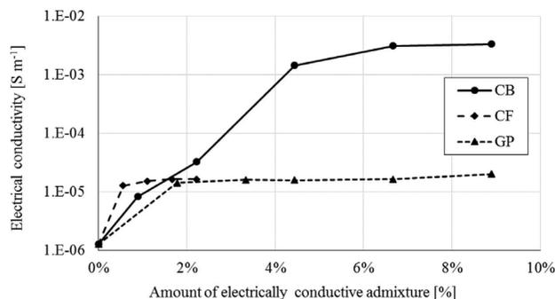
**Figure 9:** Electrical conductivity of electrically enhanced AAAs
