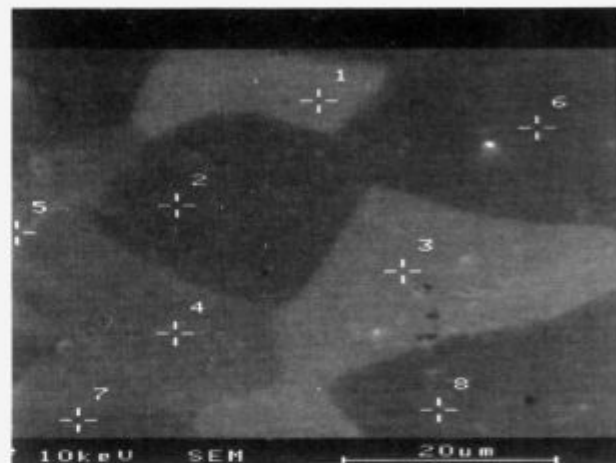
Figure 2: AES measurements of Sb surface segregation on the different grains. Antimony to iron peak height ratios for all recorded spectra are given in Table 2.
