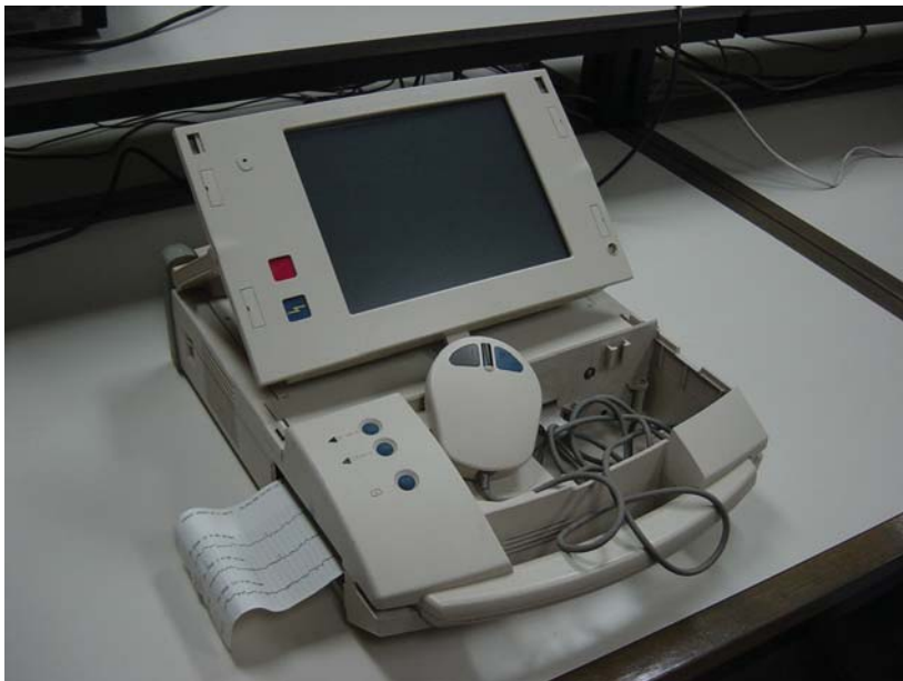
Fig. 10: Modern programmers look very much like computers and their structure indeed is very similar. The device looking like the computer mouse is the programming head to be placed over the implanted pacemaker for programming and telemetry.
