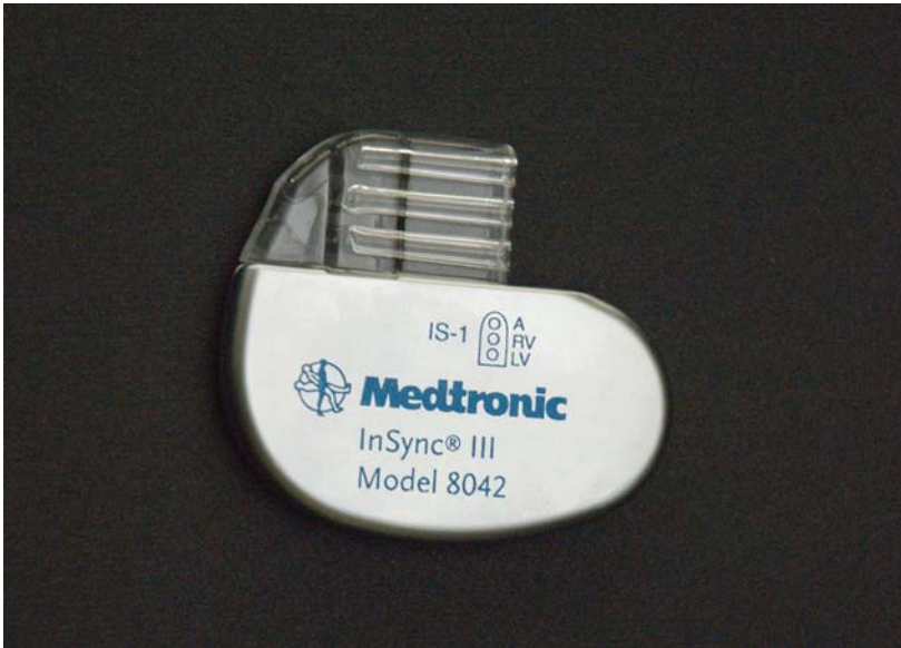
Fig. 12: Model of a biventricular pacemaker InSync III, Medtronic, 1988 (5,9x5,1x0,8 cm; 30g).
