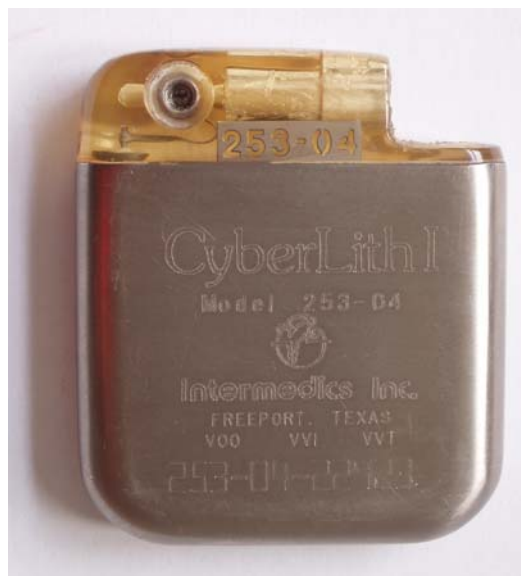
Fig. 8: CyberLith I model of implantable pacemaker, Intermedics, 1981, one of the first pacemaker models with telemetry (4,5x5,4x1cm; 60g).
