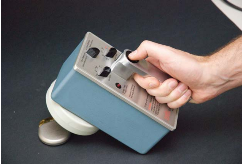
Fig. 7: Omnicor Programmer model 166B, Cordis, 1975, used for programming of early programmable pacemaker series. One of the switches was used to set the pacemaker model, and the other two for setting the amplitude and the stimulus rate. The pacemaker was (re-) programmed through the skin of the patient after implantation.
