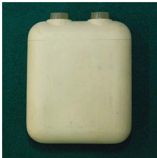
Fig. 1: a) Early General Electric pacemaker model from 1967 in plastic housing. (8x6,5x2,2cm; 200g). b) X-ray of the pacemaker. Six pieces of zinc-mercury batteries and discrete electronic components can be recognized.
