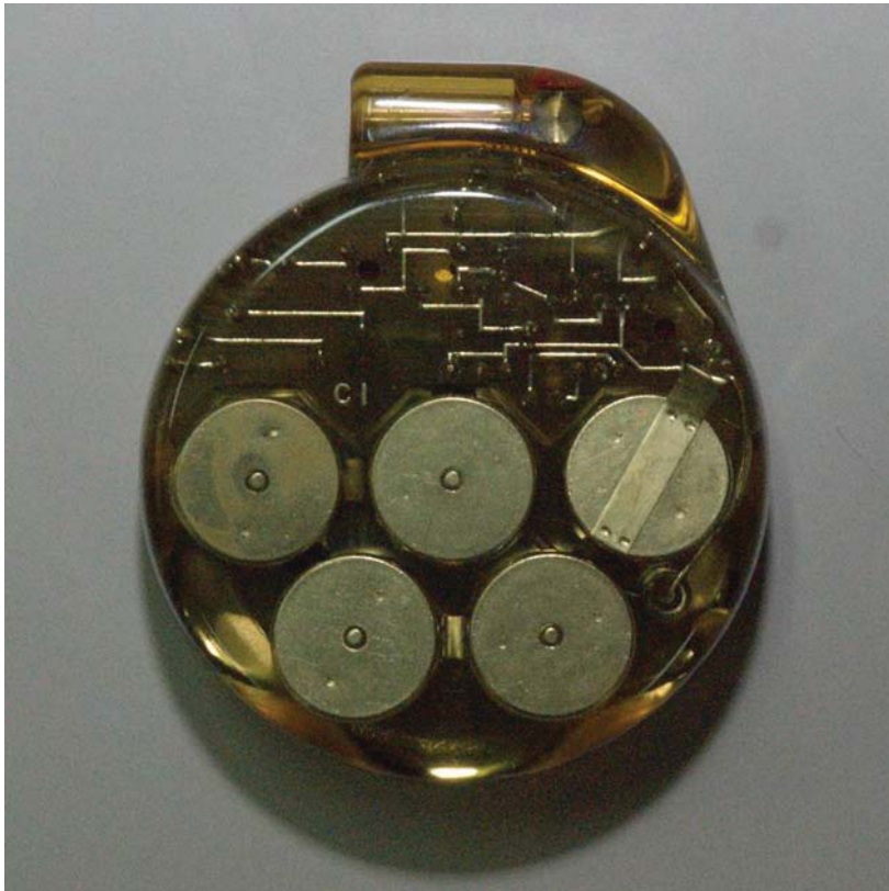
Fig. 2: Cordis implantable pacemaker, model Ectacor from 1975. The batteries and electronic circuits are sealed in epoxy resin (6,8x5,8x2,3cm; 140g)
