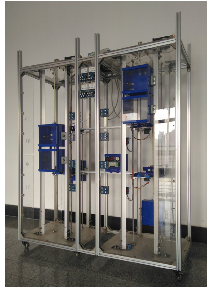
Fig. 16. Vertical and transverse elevator model
