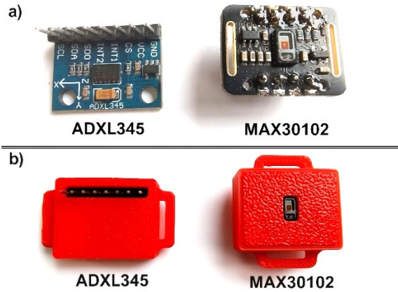
Figure 1: ADXL345 accelerometer and MAX30102 pulse oximeter a) unit modules, b) modules in 3D printed housings.
