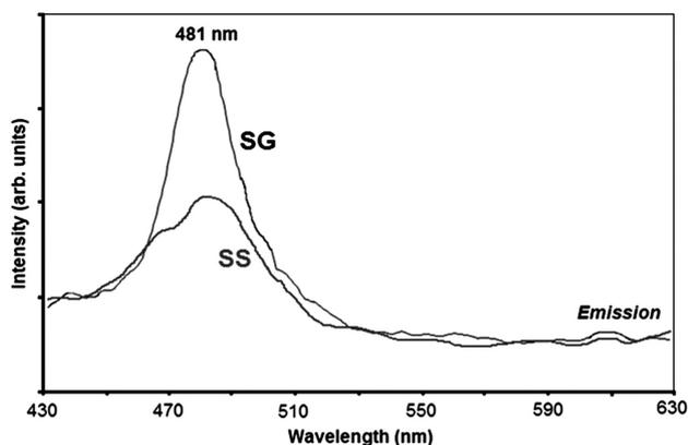
**Figure 3:** Emission spectra of  $\text{SrZn}_2\text{Si}_2\text{O}_7: \text{Eu}^{2+}$  prepared via different methods
