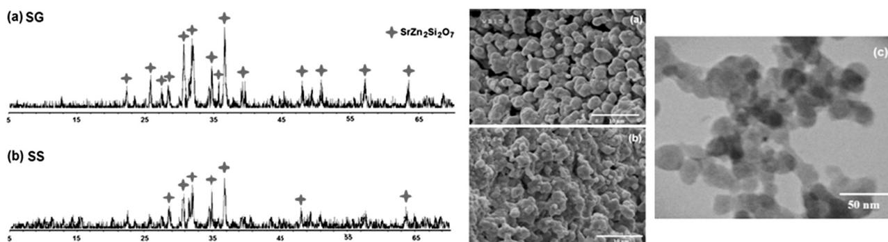
**Figure 1:** XRD patterns, SEM images and TEM micrograph of SrZn<sub>2</sub>Si<sub>2</sub>O<sub>7</sub>: Eu<sup>2+</sup> prepared via different methods
