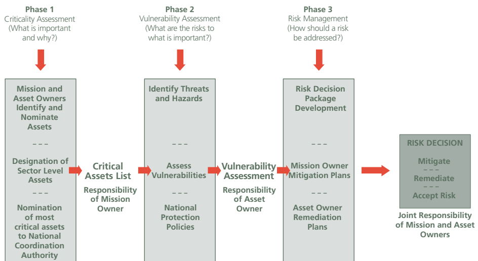
Figure 2: Mission Assurance Process (Source: Based on DISA illustration of US DoD Directive 3020.40 – Mission Assurance)
