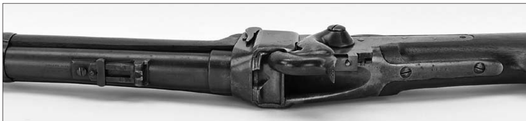
Zaklep sistema Sharps M 1859 (© Collectors Firearms).
