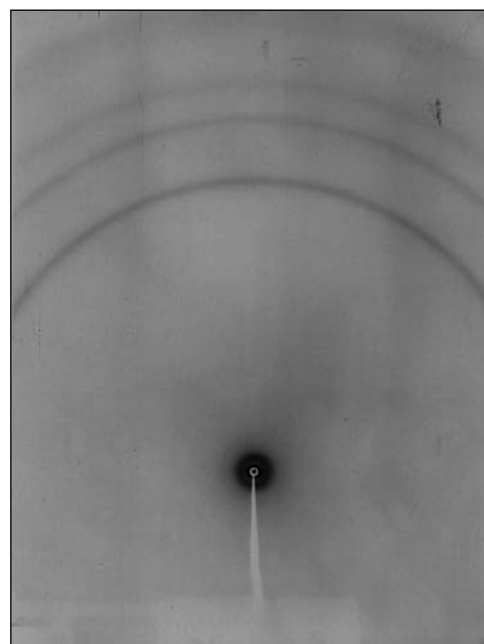
Figure 2. SAXS film pattern (fiber axis vertical) of as-spun filaments made from the plastic-grade polymer.
