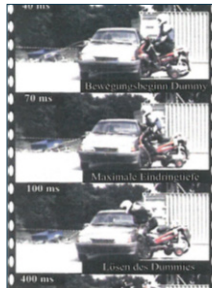
Slika 7: Crash testi, Yamaha XS850, v_1=69\text{km/h} in Ford, v_2=60\text{km/h} | Vir: Dekra. 2016; (2010)
