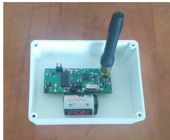
Figure 2: HW of the developed node - communication testing
