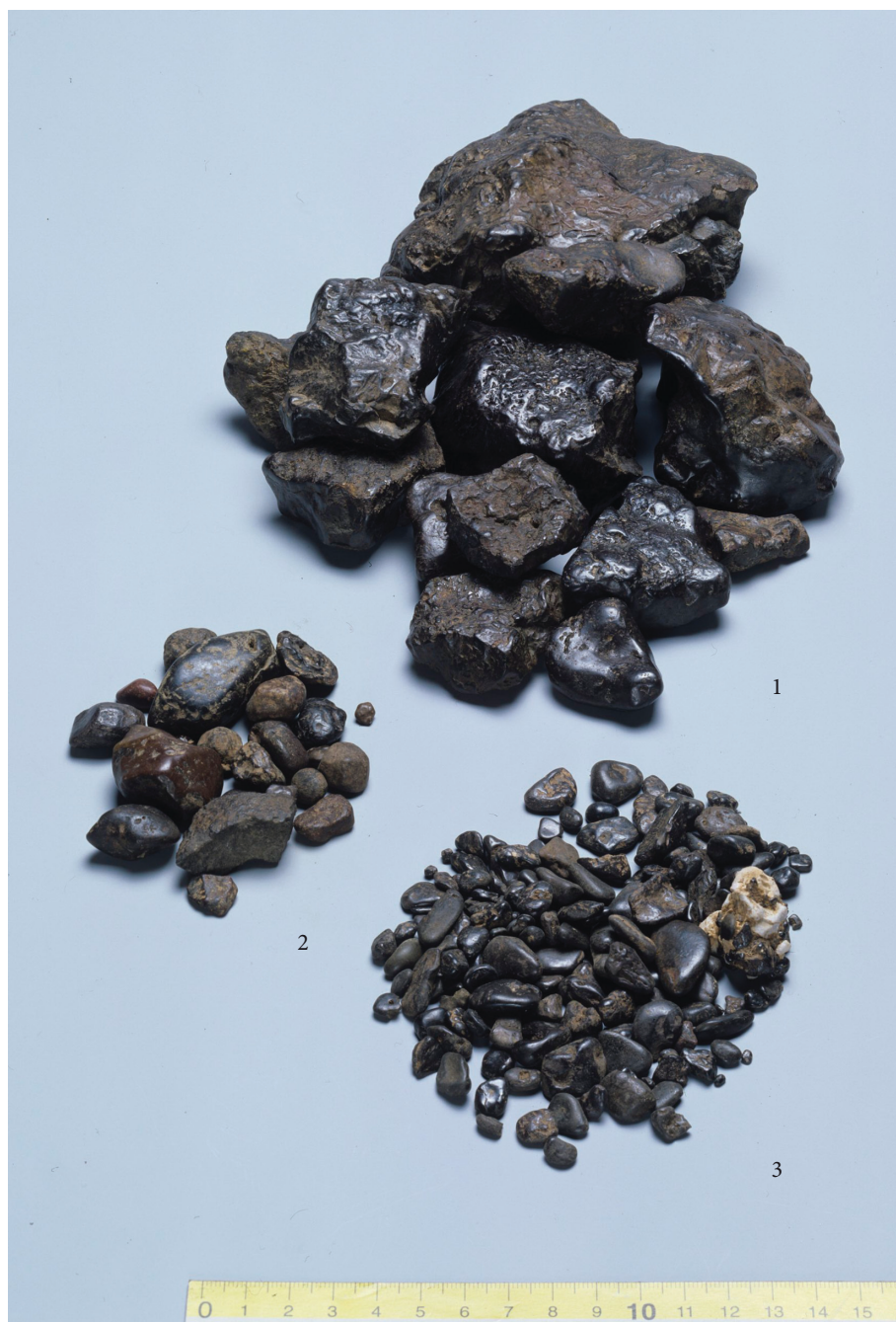
Fig.1: Iron ore – nuggets. 1 stone quarry Peči by Kamna gorica; 2 Rudno polje on Pokljuka (1,2 collected by A. Rečnik, 1999); 3 Mountain plateau of Dedno polje above Bohinj (collected by F. Stele, 1998). Photo T. Lauko.
