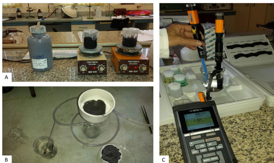
Figure 7: Chemical laboratory testing of SPL waste recovery (A mixing, B vacuum filtration, pH and conductivity measurements)
