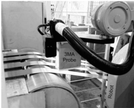
Fig. 3. Sensor attached to a robot for gradual inspection of several parallel running strips
