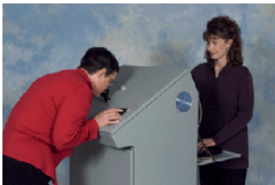
Figure 2: The AC'SCENT® International Olfactometer was designed specifically to meet all requirements of the CEN odor testing standard, EN 13725:2003 and ASTM International E679-04.
