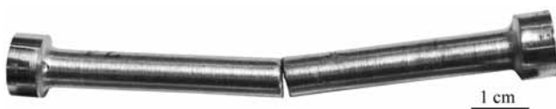
Figure 1: Macroscopic image of S 355 J2+N structural steel, showing the reduction of area specimen taken from a 90-mm heavy plate in the thickness direction
