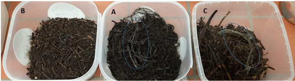
Figure 5: Composting biomass samples after 5 months of composting in piles A, B and C. The presence of the BioTHOP PLA twine is marked with ellipse.
