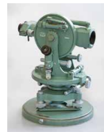
Tahimeter teodolit MOM 17 S , okoli 1940. Hrani Tehniški muzej Slovenije, Slovenska geodetska zbirka. Inv. št. / Inv. no. 800:LJU;0008638 MOM 17 S tacheometer-theodolite, about 1940. Kept at the Technical Museum of Slovenia, Slovene Geodetic Collection.
