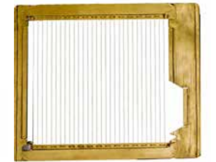
Nitni planimeter Adolf Fromme ali planimetrska harfa , okoli 1880. Hrani Tehniški muzej Slovenije, Slovenska geodetska zbirka. Inv. št. / Inv. no. 800:LJU;0008446 Adolf Fromme thread planimeter also known as harp planimeter, about 1880. Kept at the Technical Museum of Slovenia, Slovene Geodetic Collection.
