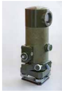
Nivelir Carl Zeiss Koni 007 , 1970. Hrani Geodetska uprava Republike Slovenije. Carl Zeiss Koni level 007, 1970. Kept at the Surveying and Mapping Authority of the Republic of Slovenia.
