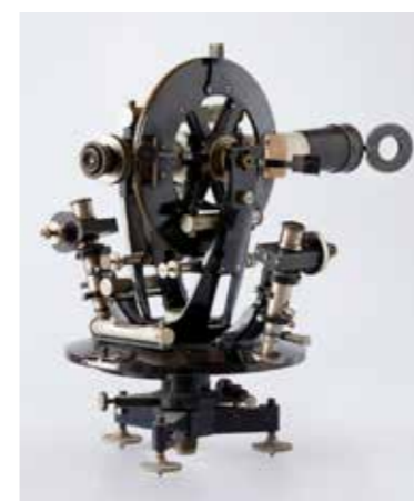
Teodolit tahimeter Ertel & Sohn , 1900 do 1910. Hrani Fakulteta za gradbeništvo in geodezijo pri Univerzi v Ljubljani (UL FGG) https://zbirka.fgg.uni-lj.si/instrument/11 Ertel & Sohn tacheometer-theodolite, 1910 to 1920. Kept at the Faculty of Civil and Geodetic Engineering, University of Ljubljana (UL FGG) https://zbirka.fgg.uni-lj.si/instrument/11.
