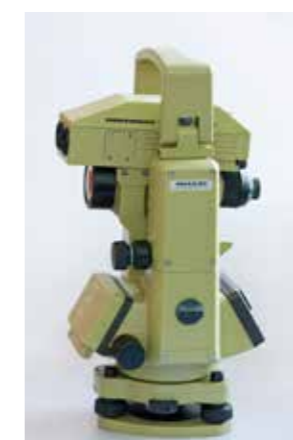
Elektronski teodolit Wild T1000 in distomat DI 1000 , 1987. Hrani Geodetska uprava Republike Slovenije. Wild T1000 electronic theodolite and DI 1000 distomat, 1987. Kept at the Surveying and Mapping Authority of the Republic of Slovenia.
