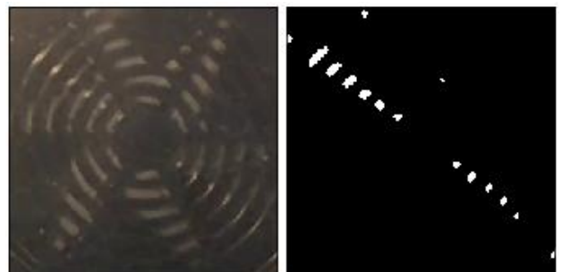
Figure 4: Original image and the obtained glare mask.
