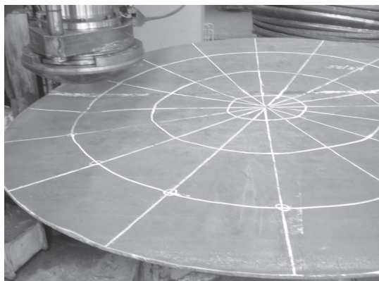
Fig.5. Incremental forming of spherical tank end
