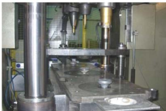
Figure 19: Three-stage tooling for barrel production.
