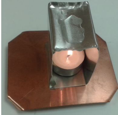
Figure 3. Evaporator for etheric oils made from copper and aluminium plates
