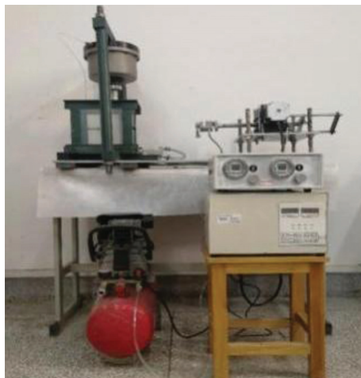
Figure 1: In-house-made pullout test equipment
