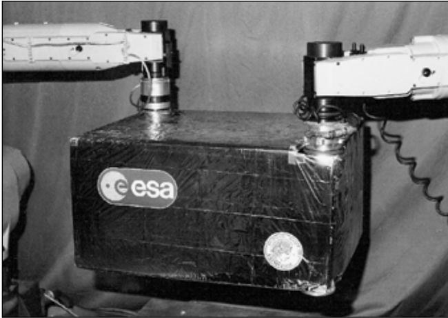
Figure 5. Handling of large Objects with Cooperative Robot Arms [12]
