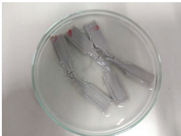
Fig. 3. Samples after 3 hours of liquid acetone treatment
