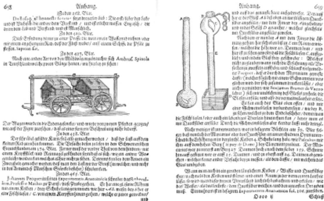
Slika 8: Schwenterjev termometer in barometer (Harsdörffer, 1651, 2: 659)
