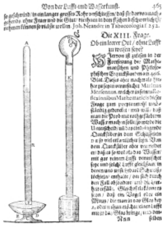
Slika 7: Schwenterjev termometer in barometer (Harsdörffer, 1651, 2: 465)
