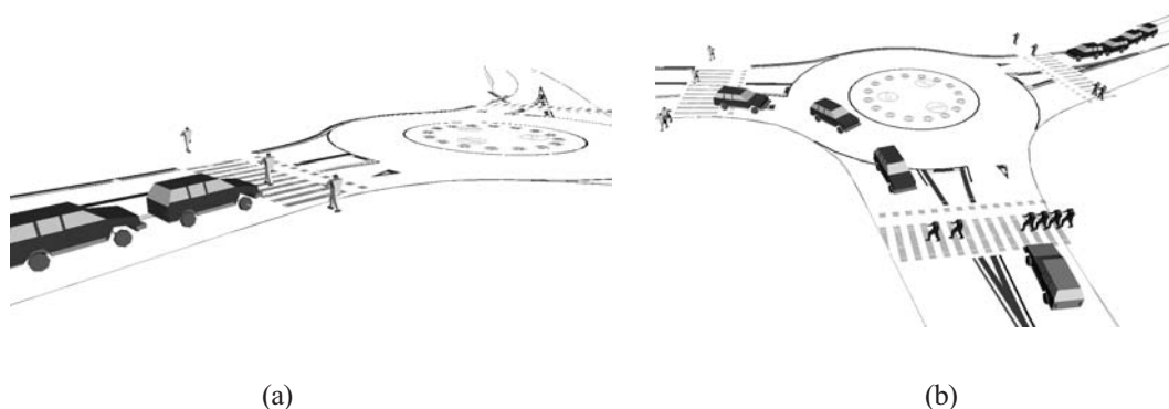
Sl. 8. Primer čakalne vrste motornih vozil zaradi toka pešcev Fig. 8. An example of a waiting line of motorised vehicles because of pedestrians' flow
