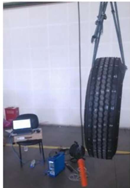
Fig. 3. Overview of tire modal test
