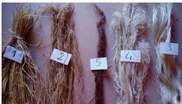
Fig. 2. Some natural fibres obtained by different methods of extraction; no. 1, 2, 5 sisal's fibres, and no. 3 and 4 juncus' fibres
