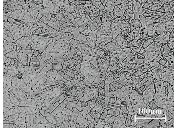
Fig. 4. Metallographic structure of 1.4301 stainless steel sheet
