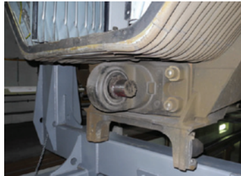
Figure 5: Bolts connected to the chassis of the second wagon of the Jacobs bogie joint
