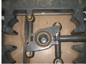
Figure 4: Slot on the Jacobs bogie where conical stud enters
