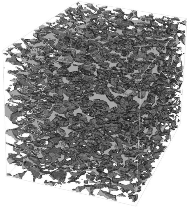
Fig. 2. 3D image ( 299 \times 300 \times 300 pixels, 0.75 \mu\text{m} pixel size) showing a specimen of the Fontainebleau sand stone.
