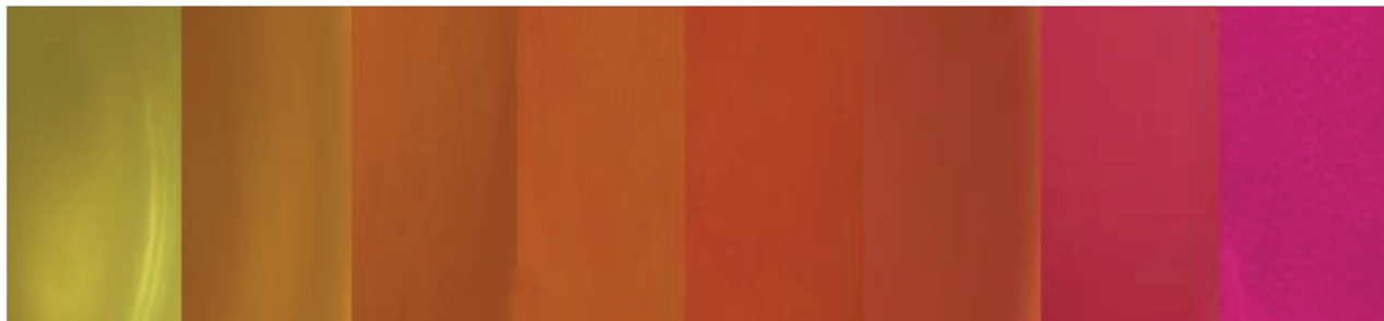
Figure 3: Color transition in the determination of the SiO 2 content by the titrimetric method
