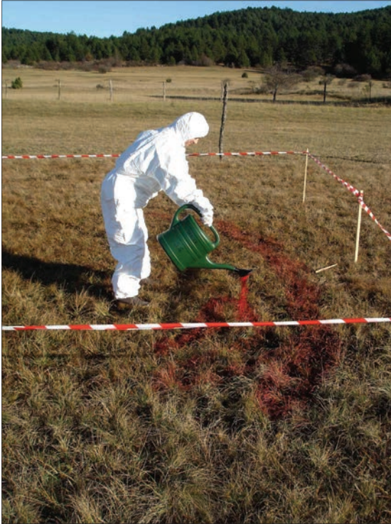
Figure 12.7: Injection of a tracer at the land surface (photo: S. Guglielmetti).
