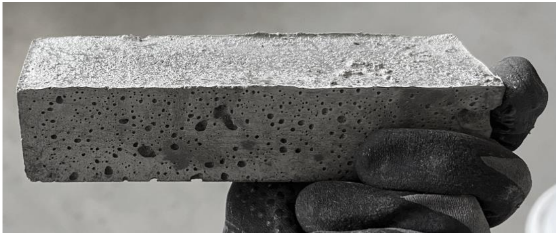
Figure 1. Specimen dimension were 40×40×160 mm applied for fatigue performance.
