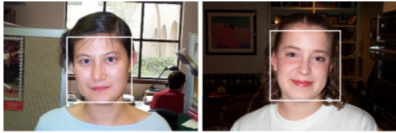
Slika 2. Zaznava obraza z Haarovimi značilkami in algoritmom AdaBoost Figure 2. Face detection using the Haar-like features and AdaBoost algorithm
