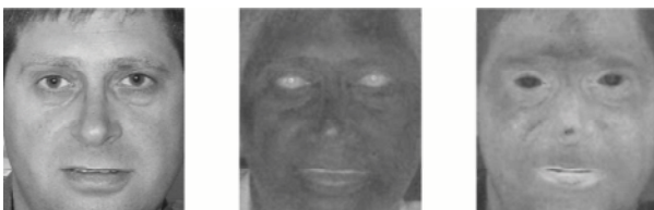
Slika 3. Komponente Y, Cb in Cr YCbCr prostora Figure 3. Y, Cb, Cr components of the YCbCr color space
