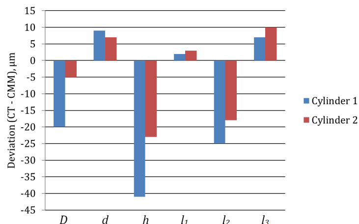
Fig. 7 Deviation between CT and CMM results for cylinder 1 and cylinder 2
