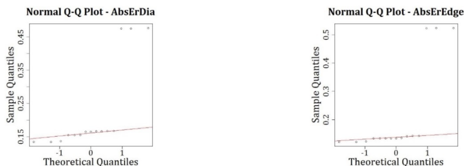
Fig. 2 Absolute error deviations for diameter (left) and for edge length (right)
