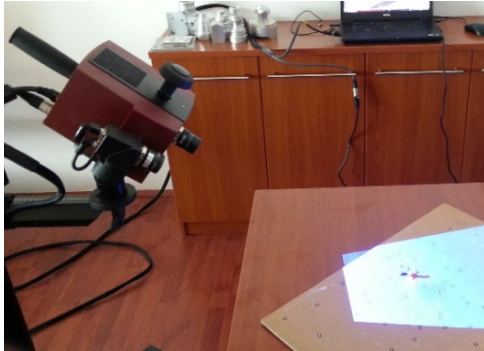
Fig. 2 Scanning kidney stone with ATOS Compact Scan
