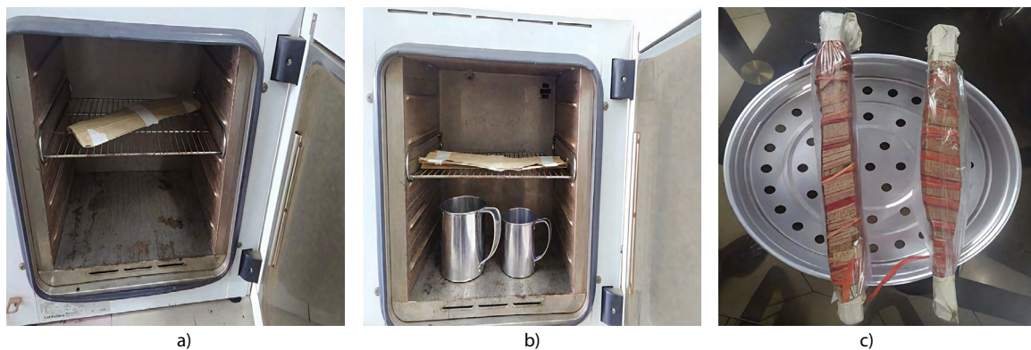
Figure 3: Permanent pleating process a) oven drying b) oven drying with water mugs c) steaming
